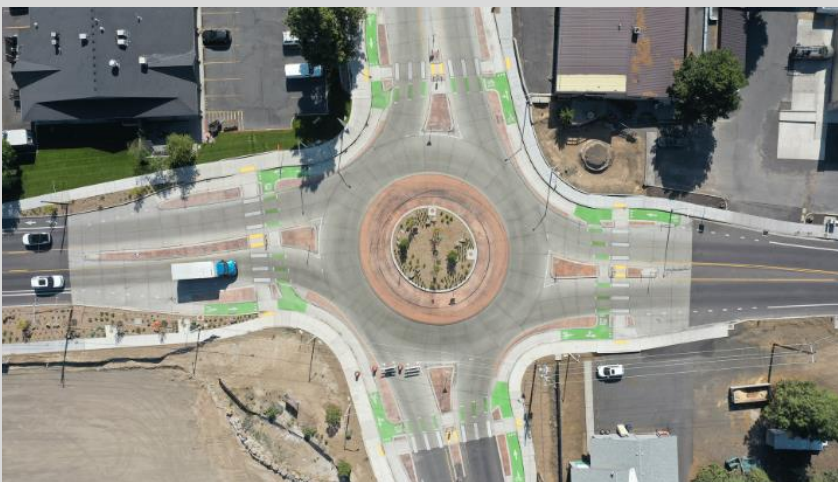
Figure 4-29 Roundabout with Separated Pedestrian and Bicycle Facilities in Bend, OR (Suburban Context)
